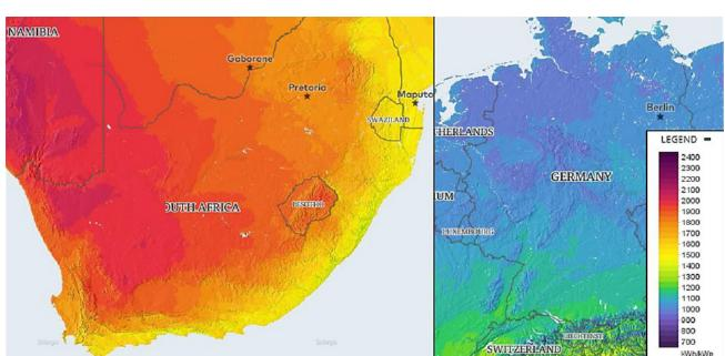
Figure 17: Comparison of the solar PV production potential in South Africa and Germany. Source: Wright et al. (2017)..
